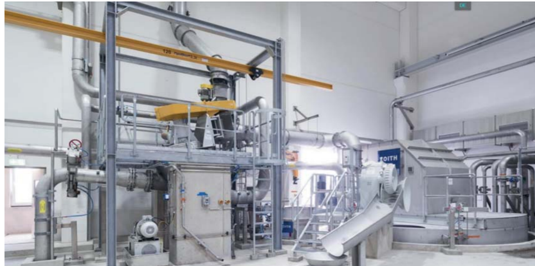
The TwinPulp system prevents unnecessary shredding of impurities by early and consistently removing coarse contaminants. This relieves the whole downstream process and contributes to cleanliness at this early stage
