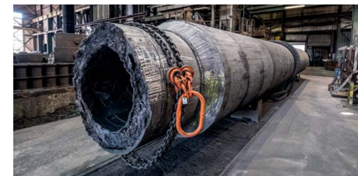
The calender rolls for Papierfabrik Palm are made from 76-tonne castings
