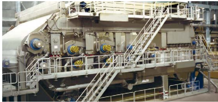
A Twin Wire Press of the type that ANDRITZ will supply to Guangxi Sun Paper's new pulp mill in China
