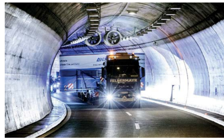
Based on the ANDRITZ engineering and logistics concept, the Yankee was transported in two halves and assembled on site
