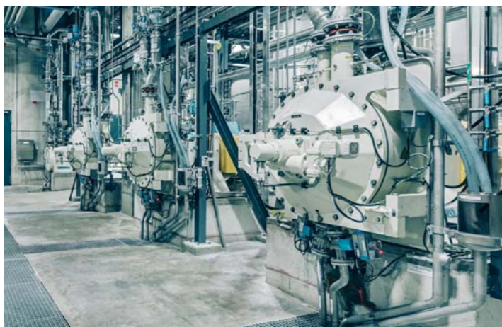
Five TwinFlo disc refiners enable smooth and efficient refining
